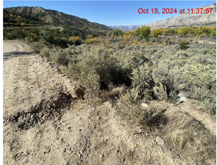
Insufficient Erosion Control/Sediment Transport from Lease Road – Photo #04238
