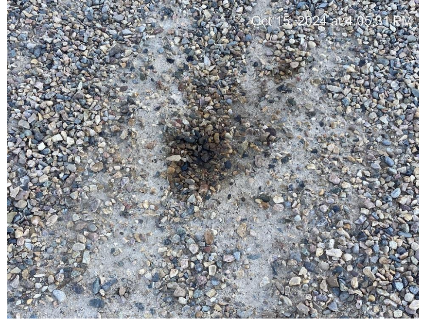
Staining outside of tank berm
