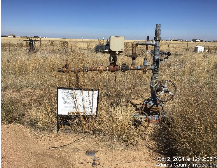
Photo #5 Well head (weeds throughout location).
