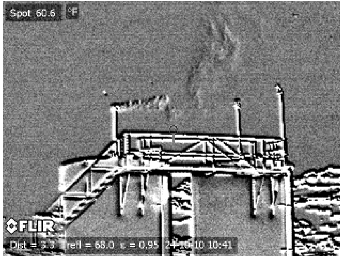
FLIR video of leaking enardo valve on tank battery.
