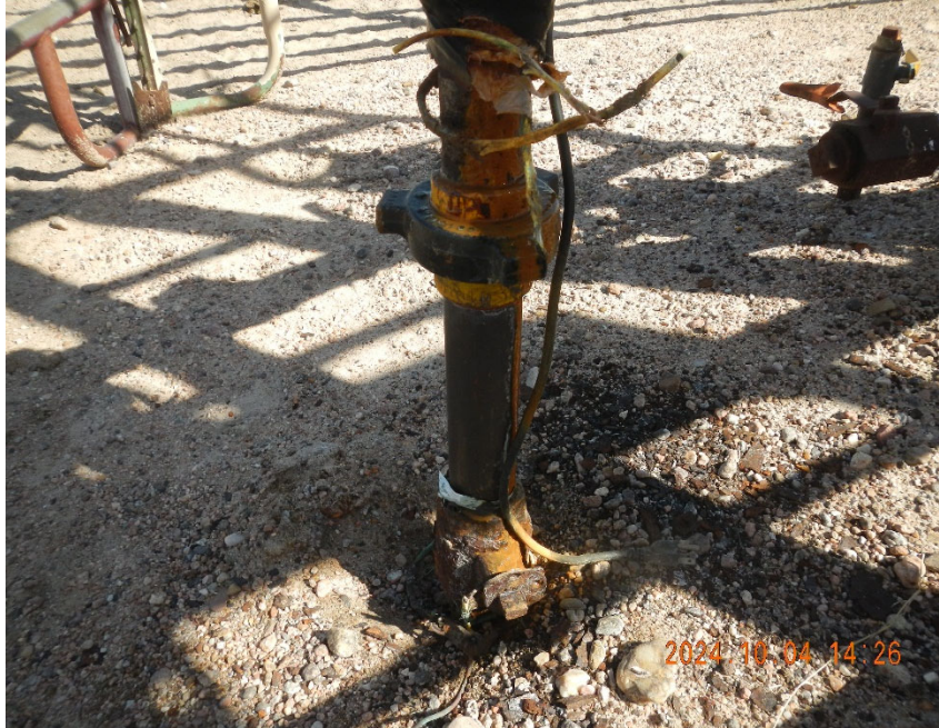
3. View of water leg hammer union.
