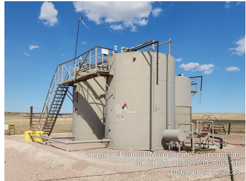
Photo 6 – Tank Battery
