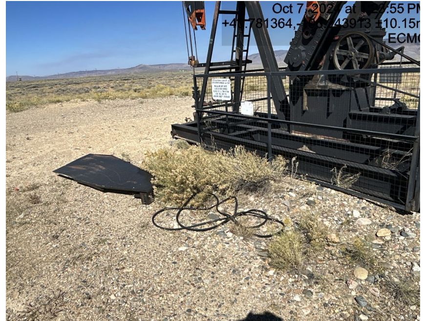
Belt guard and debris
