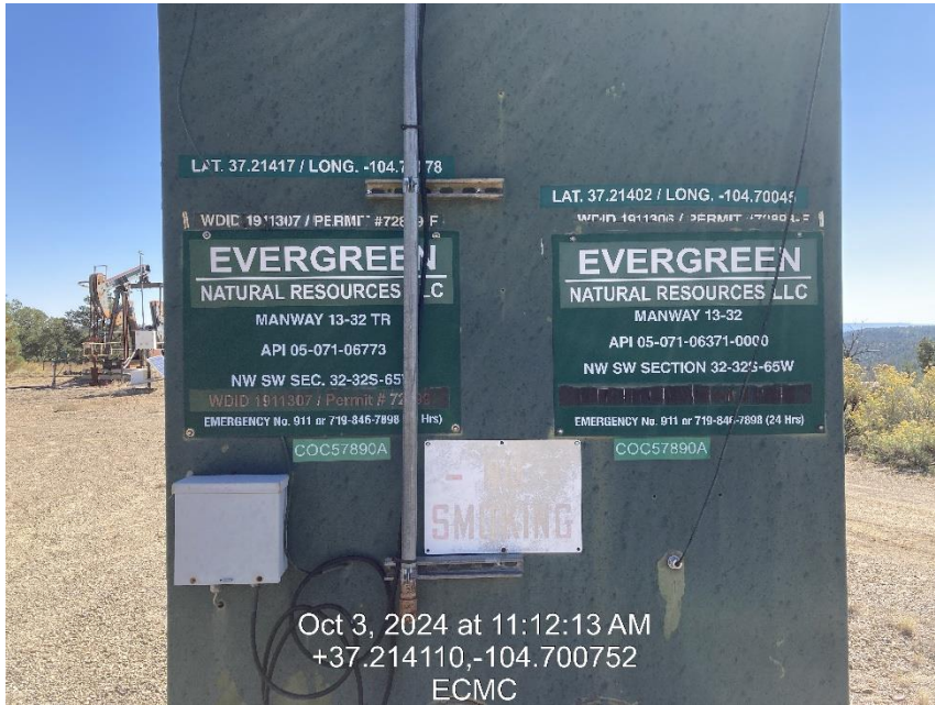
Photo 1 – Well placard on meter house, WDID stickers illegible
