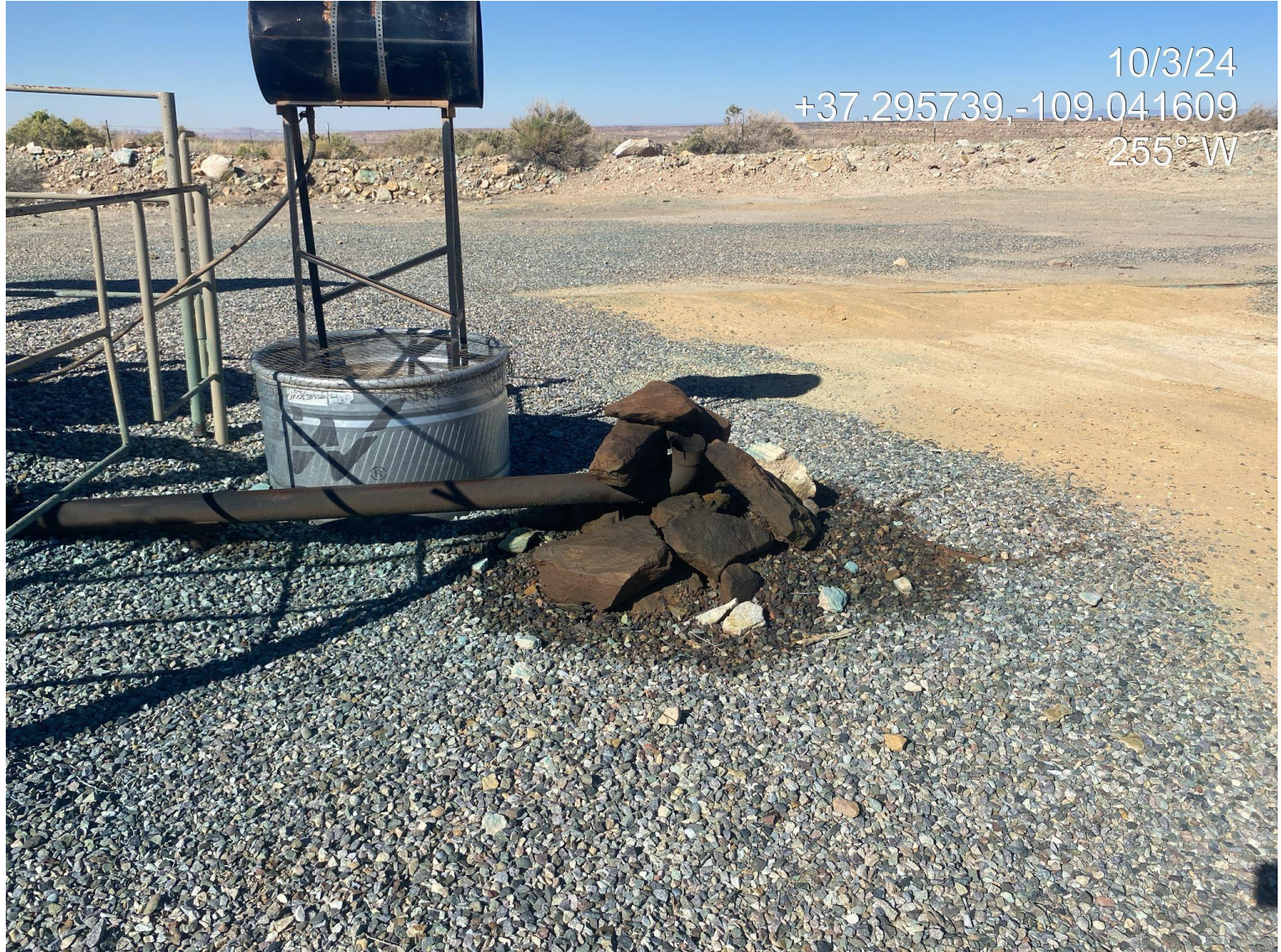
Photo 2. Stained soils observed at pump jack muffer.
