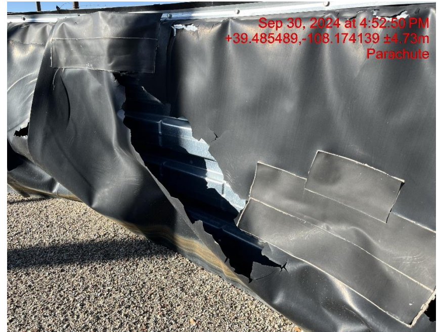
Holes in secondary containment liner - Photo #06640
