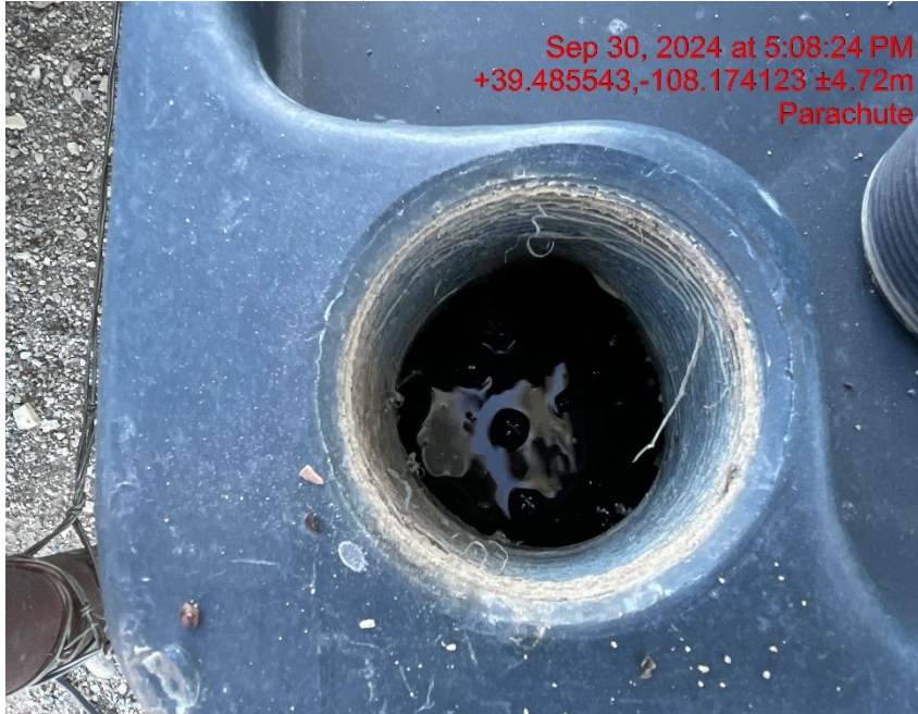
Failure to maintain chemical BMP/chemical tank containment \frac{3}{4} full of fluid - Photo #06665
