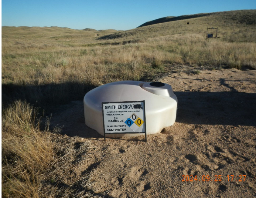
5. View of produced water tank.
