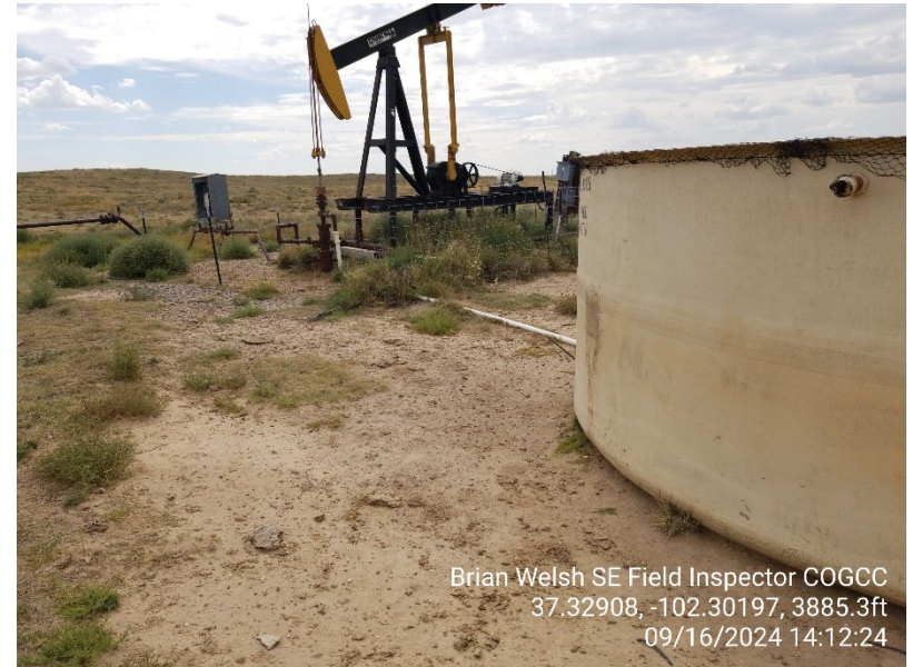
2. Water tank has no berms. Meter run on south side of wellhead
