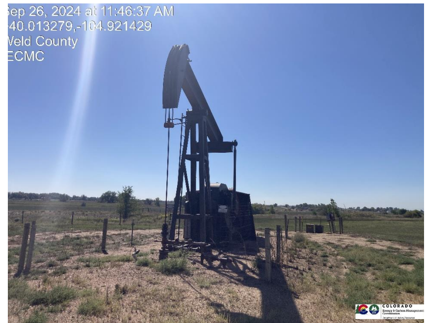
Pic 6 Wellhead pump jack
