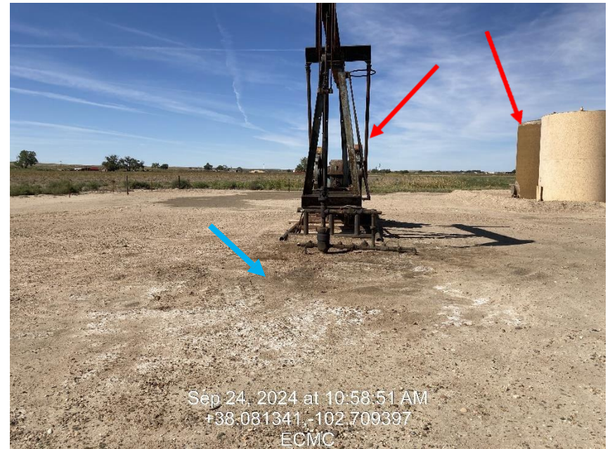
Photo 2 – Wellhead and equipment, Impacted soils at blue arrow
