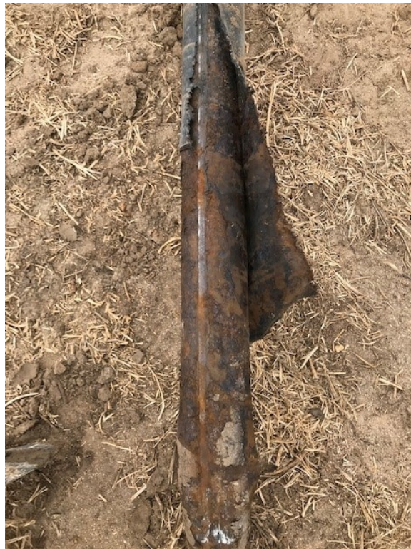
#10 – Inspection of 2" Steel Flowline; Light Corrosion, No Failures
