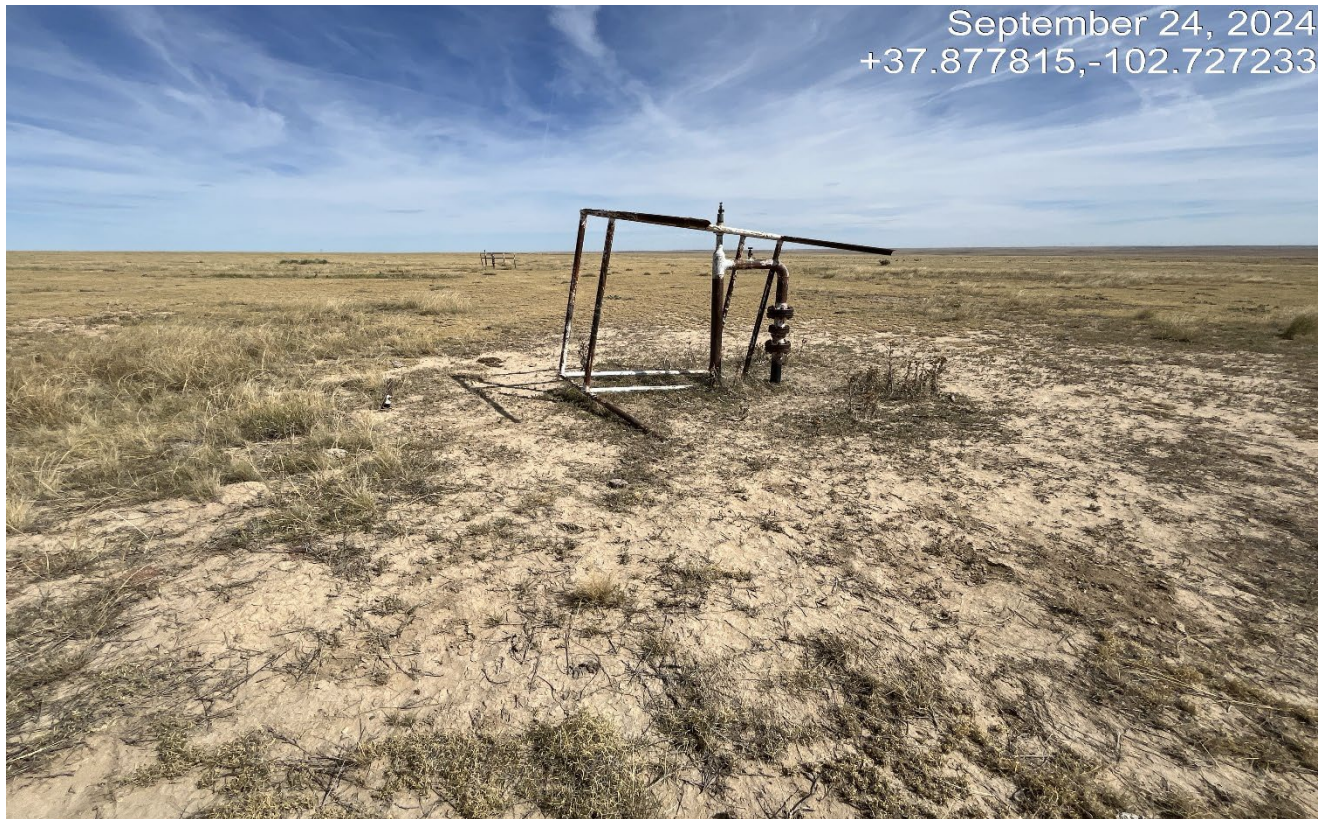
Photo 3. Facing east at the location. There are two pipe risers that remain at the location shown at red arrows. Vegetation has not re-established near the risers.
