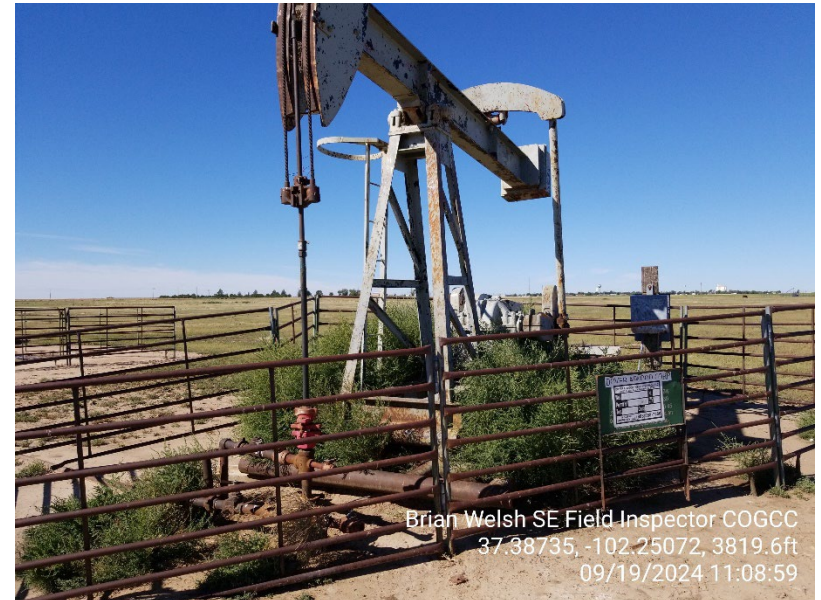
2. Pumping unit and wellhead
