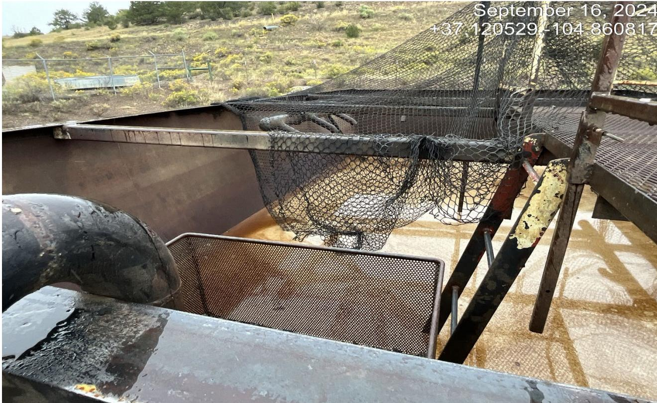
**Photo 5.** The netting on the open top tank does not cover the entire open top tank. Previous CA was not completed.
