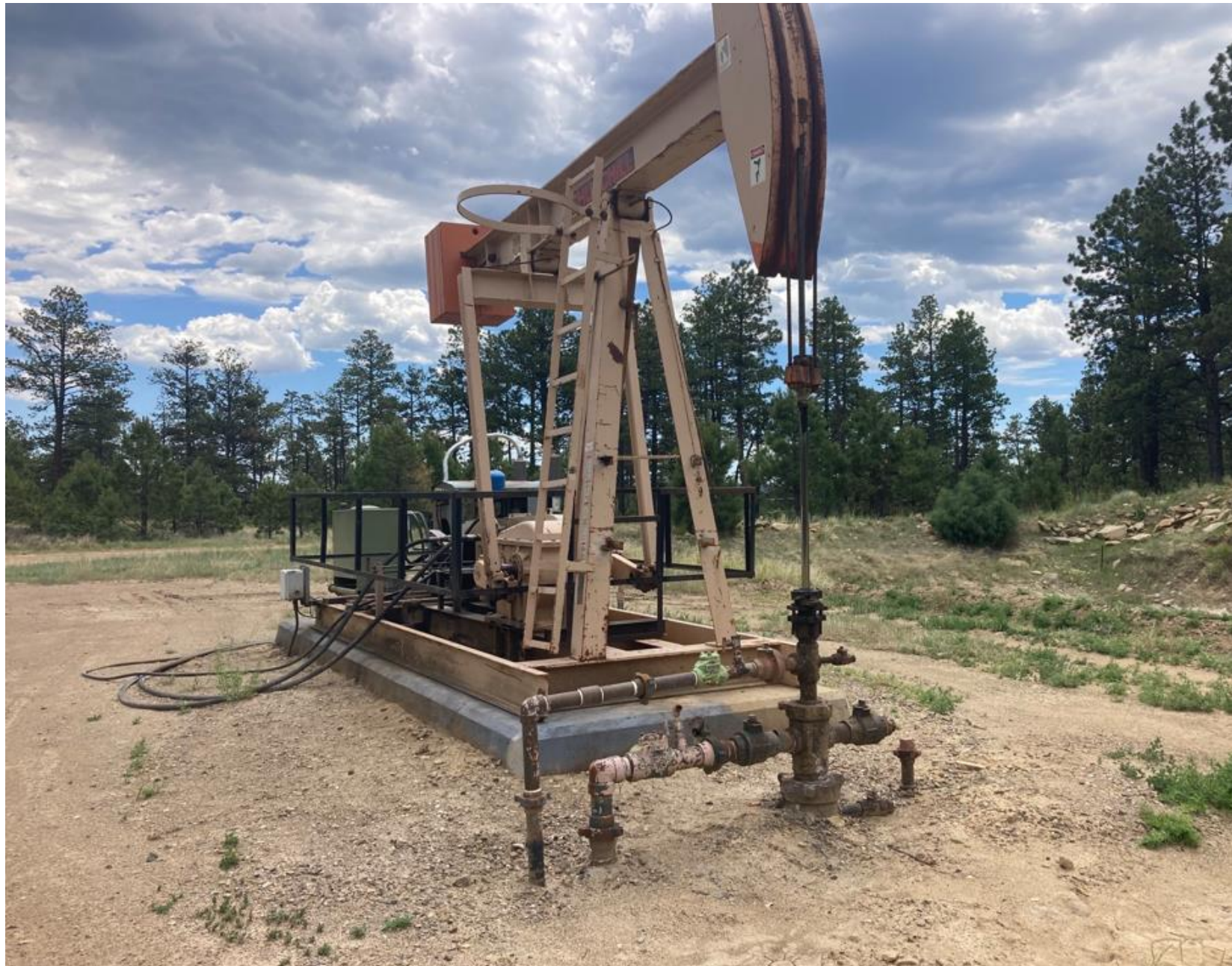
PHOTO 3: MECHANICAL MAINTENANCE HAS BEEN PERFORMED ON THE LEAKING GEARBOX AT THE PUMPJACK AND THE SKID HAS BEEN CLEANED OF ANY OIL.
