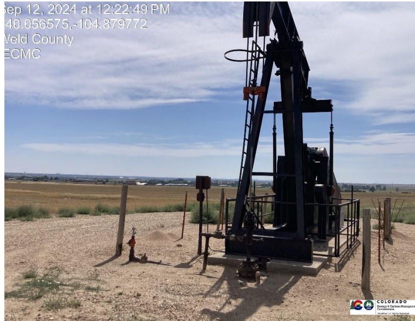
Pic 1 wellhead / pumpjack
