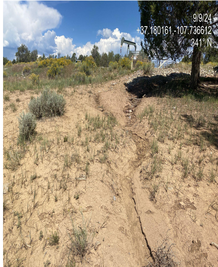
Photo 2. View of erosion observed forming in the southern interim reclamation area.
