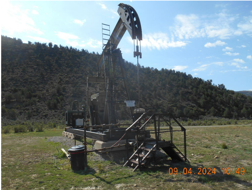
Wellhead with pumpjack
