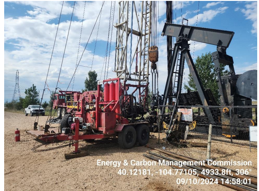
Photo 2 Accumulator, WO rig & pump jack.
