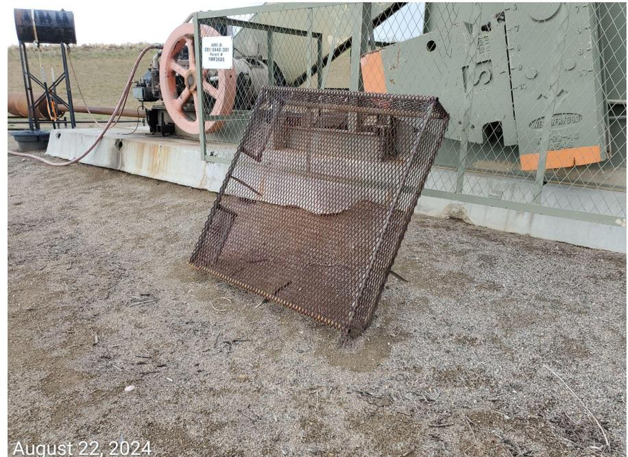
**Photo 10:** Photo left taken during the 5/8/2023 inspection. Inspection noted that the guard was not installed on the pumpjack. Operator submitted a Resolution stating guard was replaced. Photo right taken 8/22/2024 and show guard remains improperly stored, and has not been replaced.
