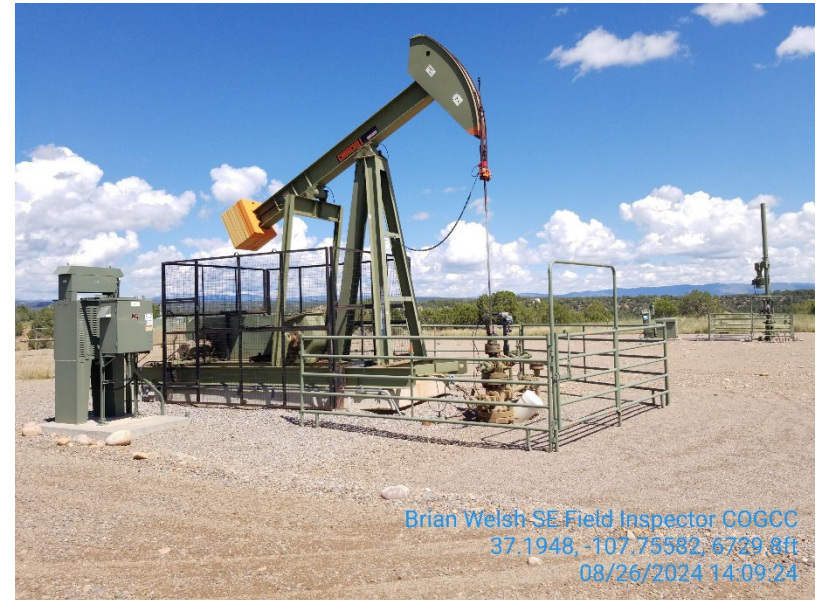
2. Pumping unit and linear rod pump
