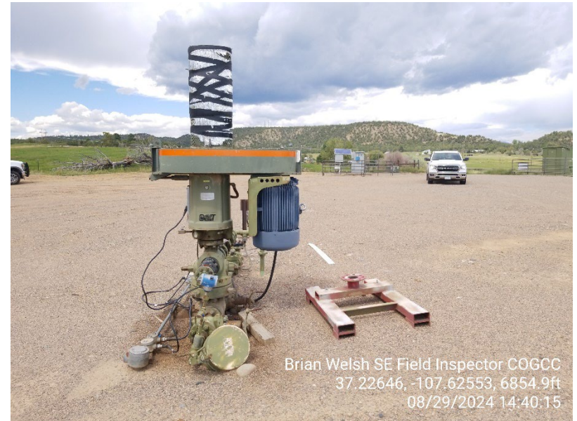
2. Progressive cavity on wellhead
