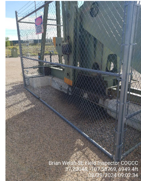
4. Stained soil at base of pumping unit
