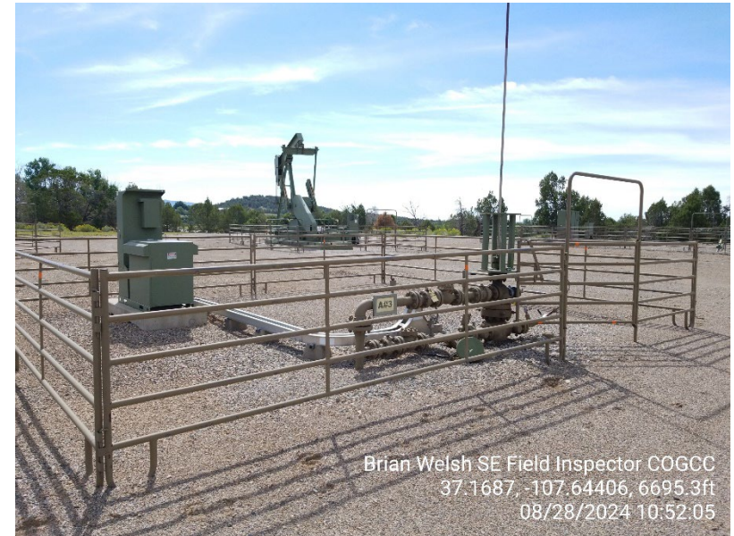
2. James A 3 wellhead and control panel
