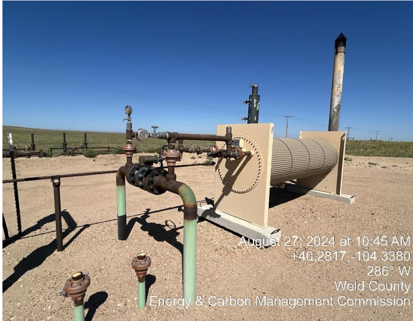
Line heater and unmarked risers
