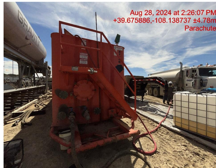
No labeling on Frac tank/Diesel tank - Photo #05161
