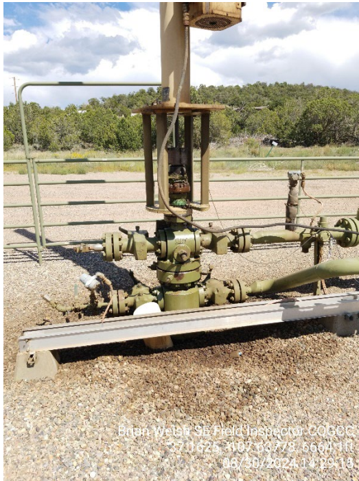
3. Gary Patrick 2 wellhead and pump. Remove and remediate stained rock and soil around wellhead
