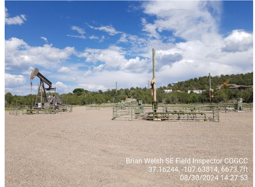
2. Pumping unit and linear pumps
