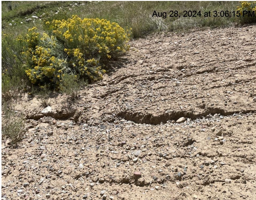
Photo # 7176 Erosion on slope & transport of sediment off location & into a vegetated area (near separator units & Summit Midstream meter house)
