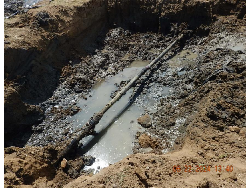
Failed flowline segment exposed in excavation. Note: Corrosion pinhole is above ripple in water (7 o'clock)
