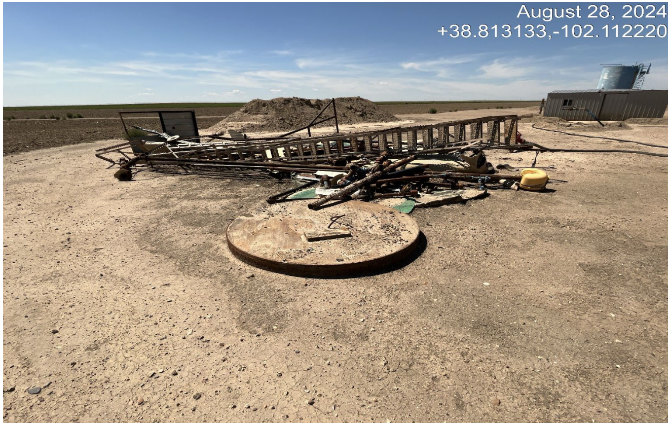
Photo 2. There is unused equipment on location with rusted out flowlines and a burnt fiberglass tank.
