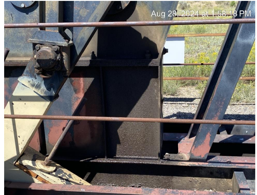
Equipment leak. Oily waste and stained soil below
