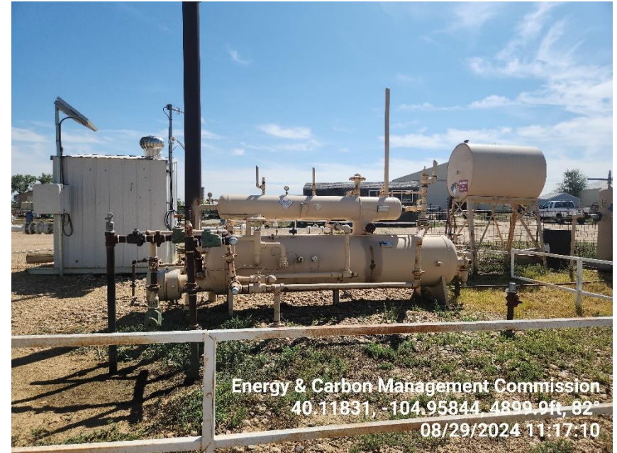
Photo 6 Horizontal Heated Separator SI, LOTO
