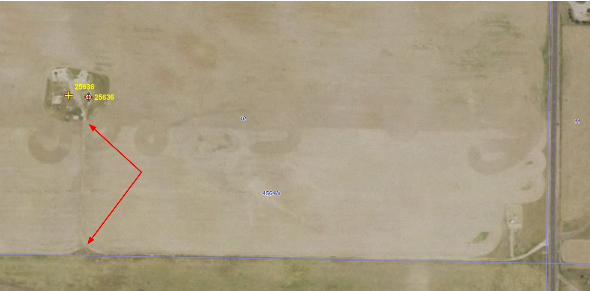
Photo 1. 2021 aerial imagery illustrates a portion of the access road between the red arrows where gravel has not been removed; therefore, decompaction has not been performed. Refer to Photo #2. In addition, the location has not been recontoured and decompaction has not been performed.
