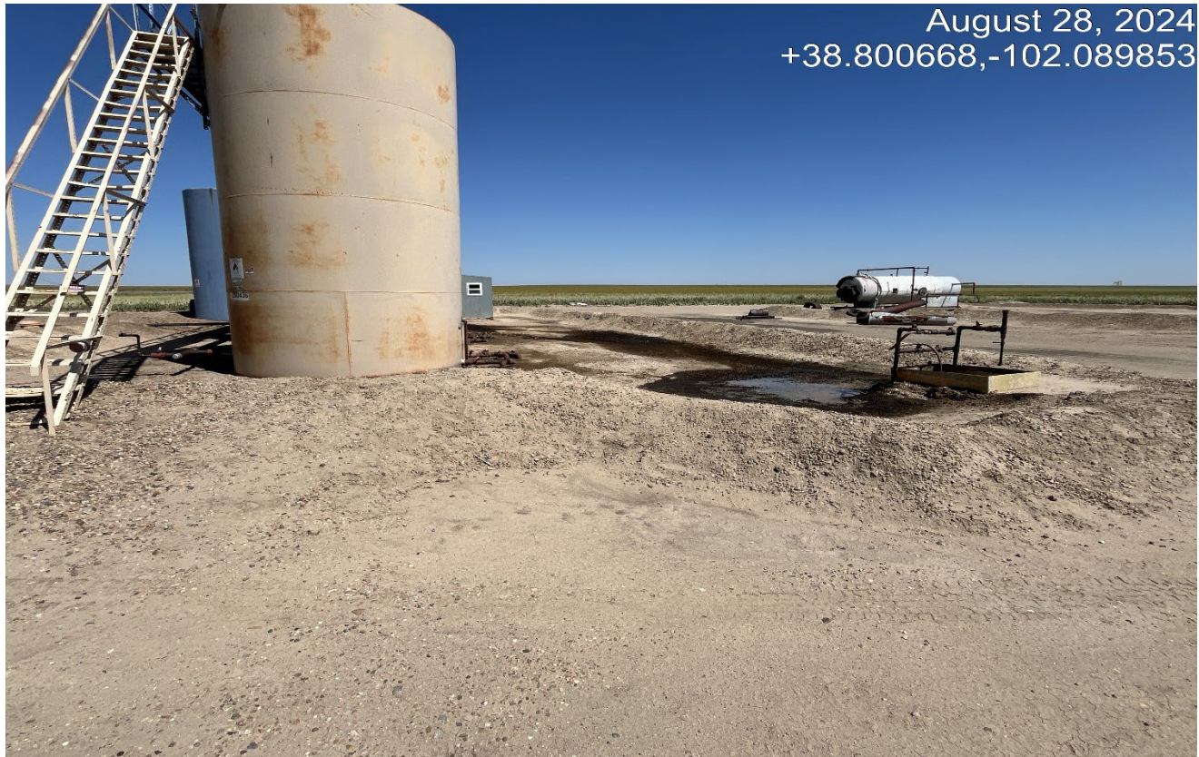
Photo 3. Facing northeast at the tank battery. There are stained soils from a spill that occurred at the backside of the tanks. The spill was contained in the secondary containment..
