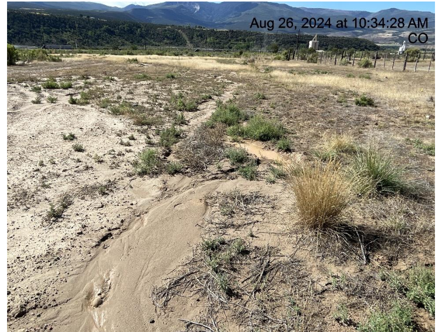
Photo # 6456 Erosion & transport of sediment off location & into a vegetated area/failure to minimize erosion & transport of sediment
