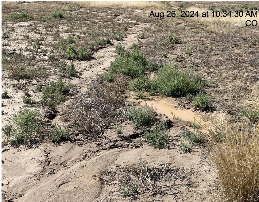
Photo # 6457 Erosion & transport of sediment off location & into a vegetated area/failure to minimize erosion & transport of sediment
