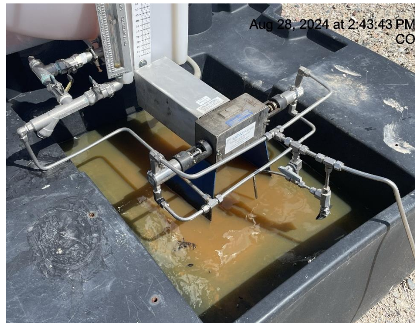
Photo # 7117 Failure to maintain chemical BMP - Chemical tank containment approximately 3/4 full of fluid/BMP insufficient to contain possible spill. (Standing fluid on chemical containment is also a wildlife hazard)
