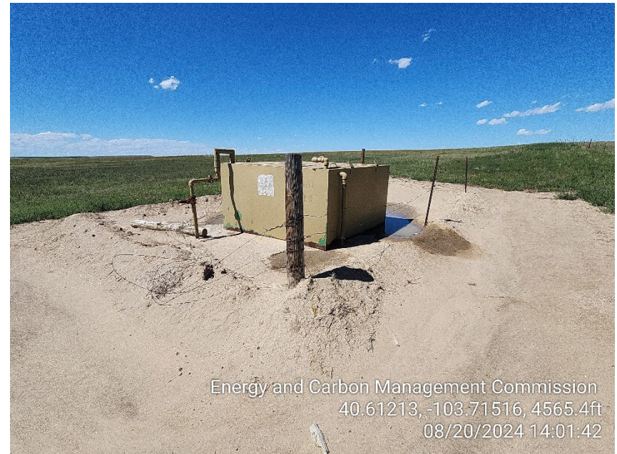
Photo 6 – Berms Inadequate
