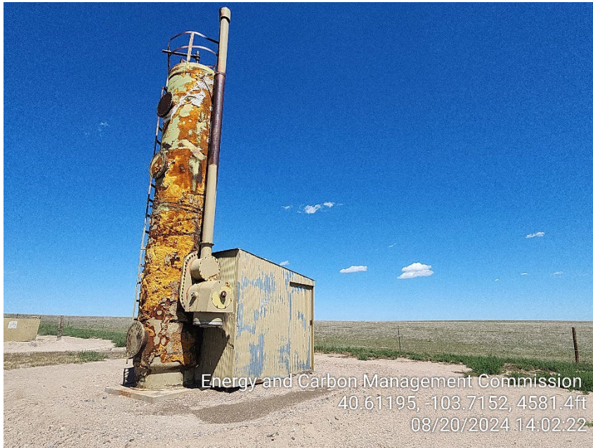
Photo 9 – Heater Treater
