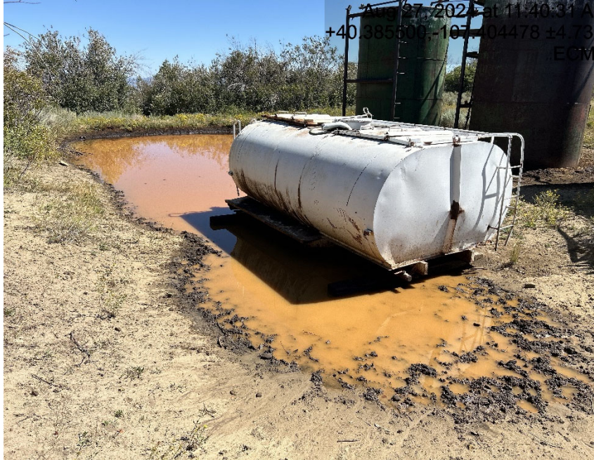
Oil and stained materials in secondary containment. Unknown tank
