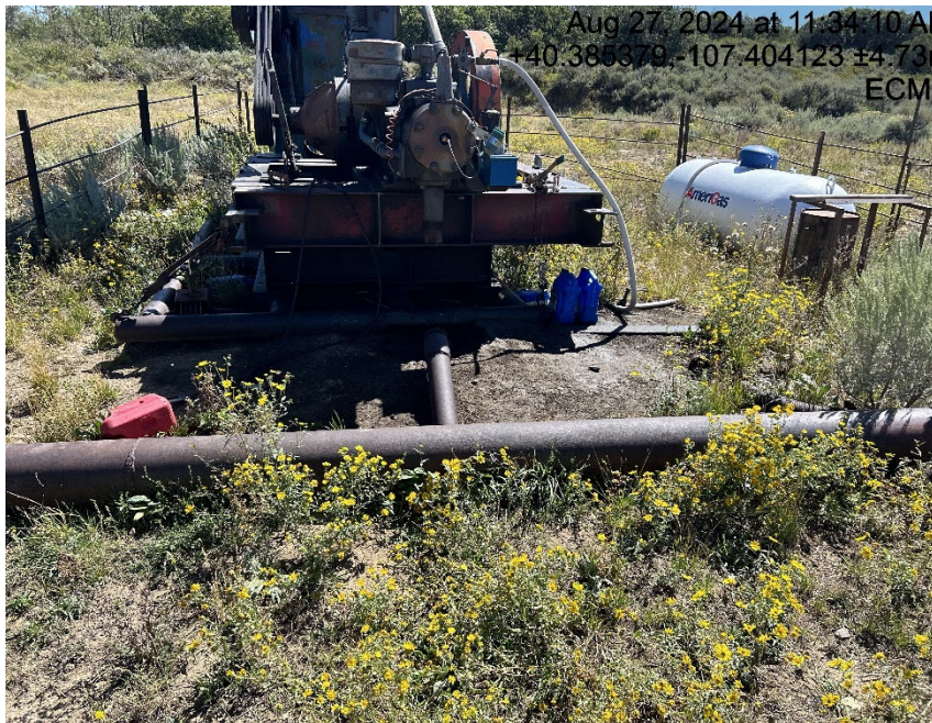
Weeds, trash, debris, staining under exhaust
