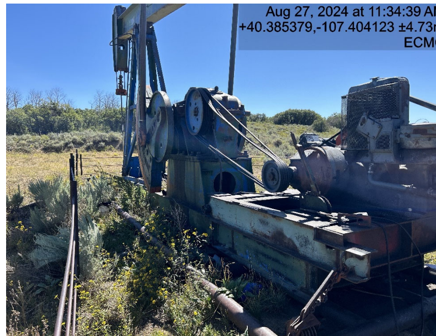
Belt guard is missing
