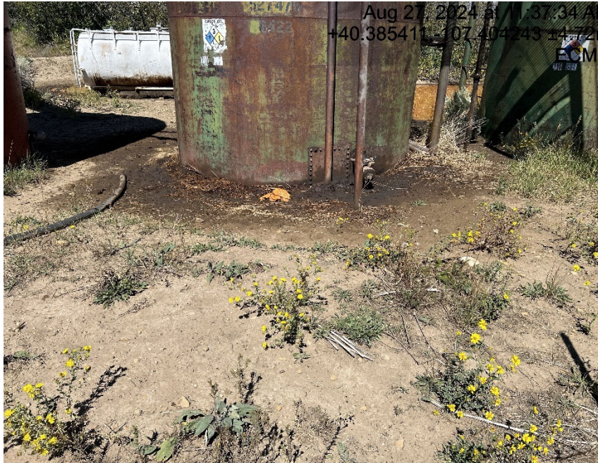
Oil and stained materials in secondary containment. Open load lines
