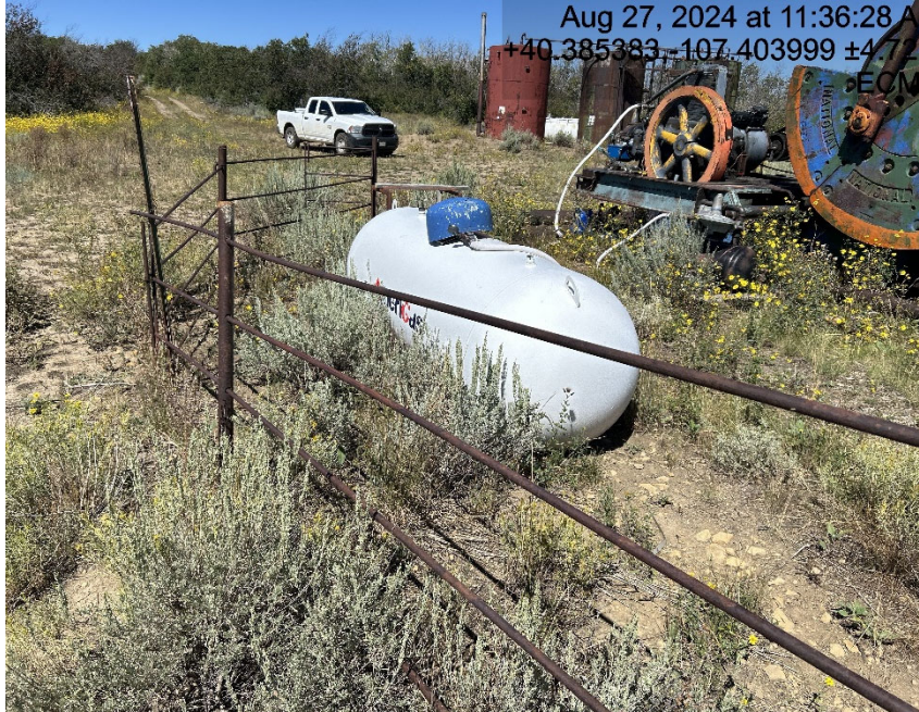
Debris, weeds around equipment, propane tank not labeled
