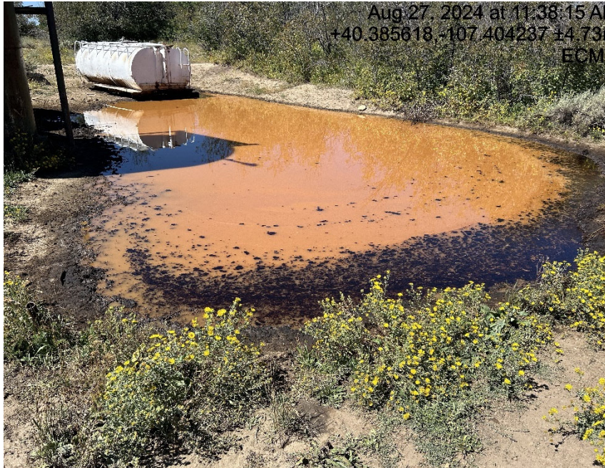
Oil and stained materials in secondary containment
