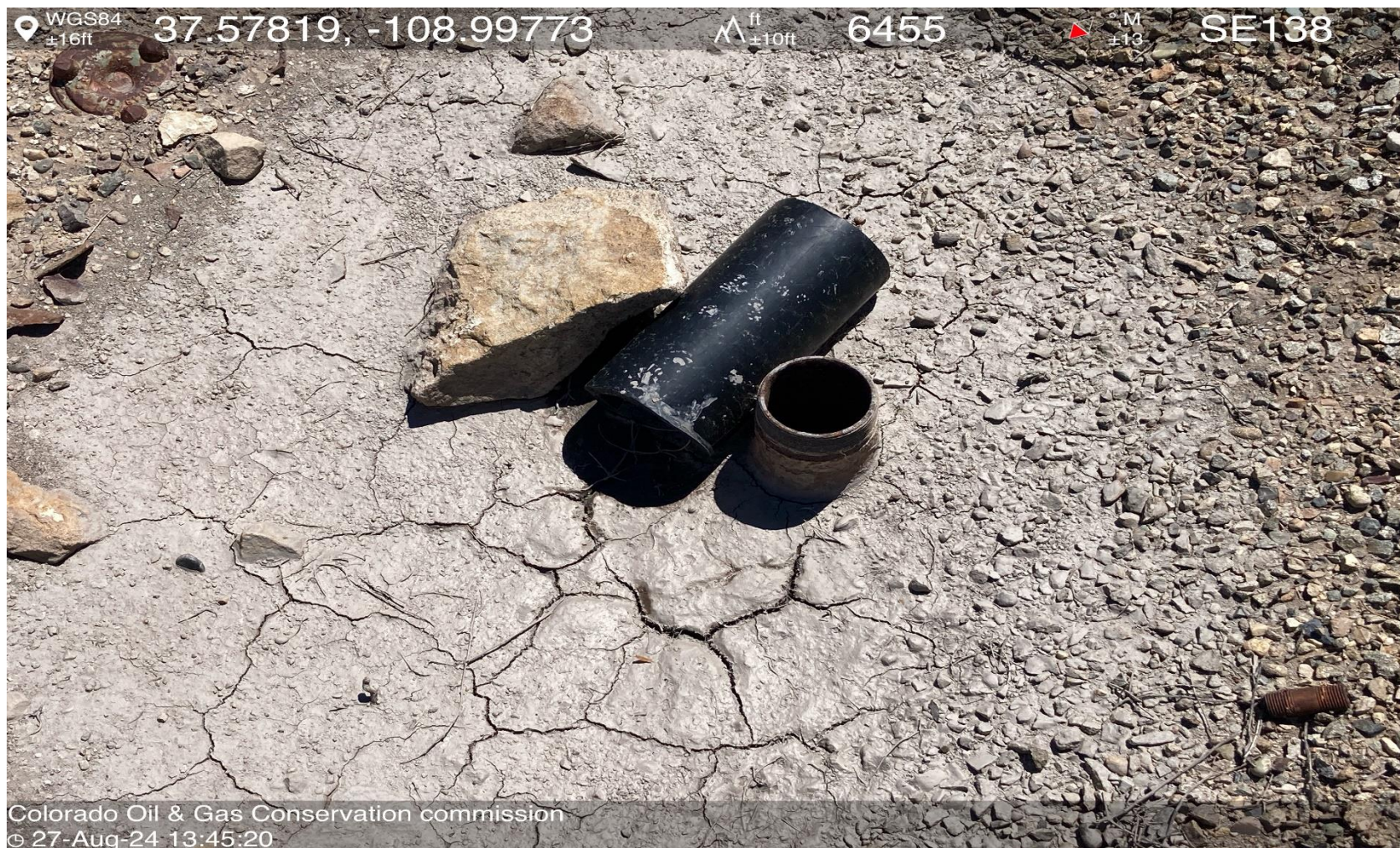
PHOTO 10: UNUSED EQUIPMENT (1 3" RISER NEAR PRODUCED WATER TANKS). REMOVE OR MARK RISERS FOR WHAT THEY CARRY (IE. WATER, GAS ECT.). PER RULE 606.
