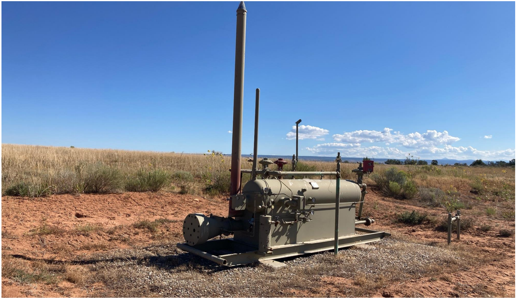
PHOTO 5: HEATED SEPARATOR
