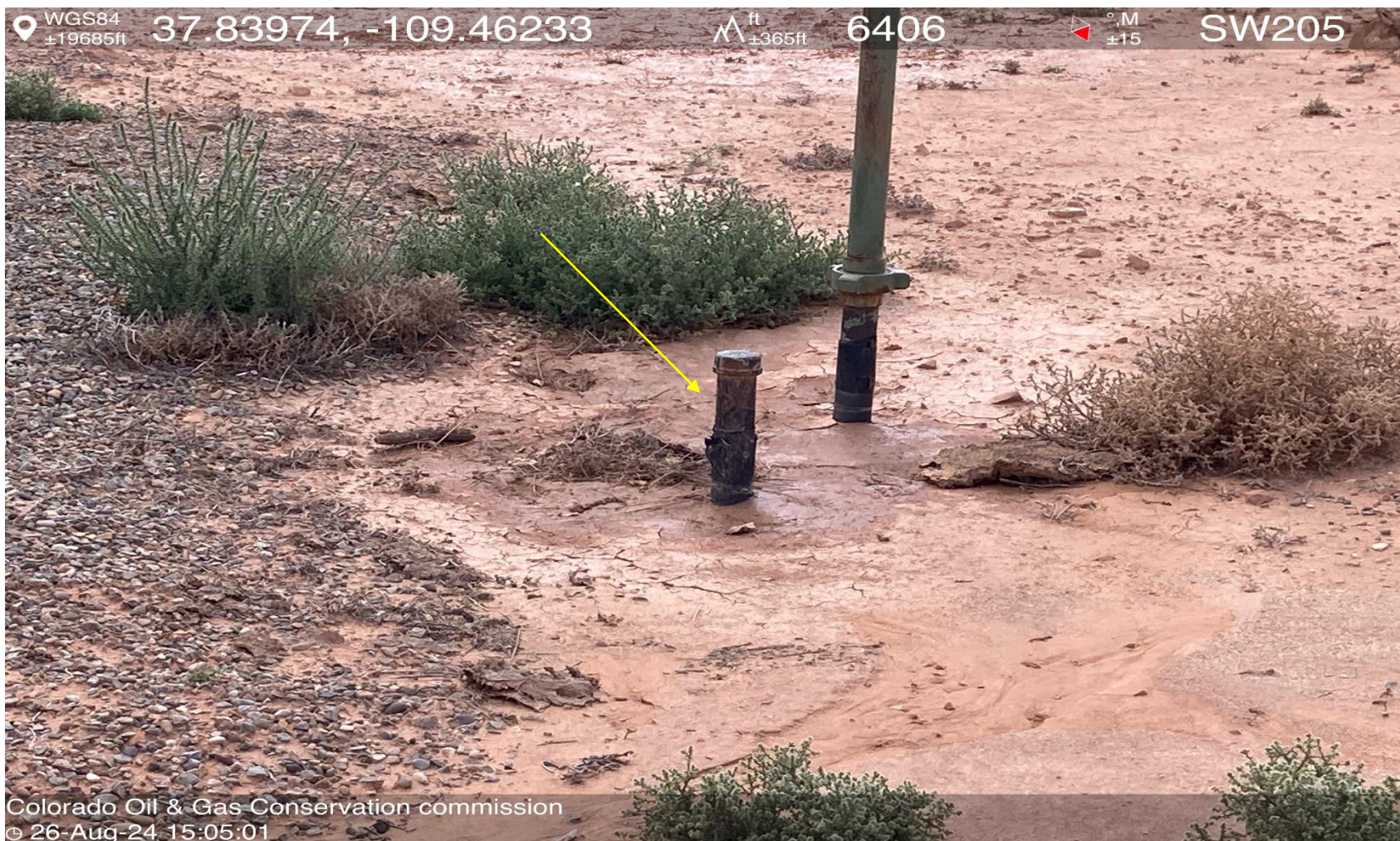
PHOTO 6: UNUSED EQUIPMENT (RISER). REMOVE UNUSED RISERS PER RULE 606.
