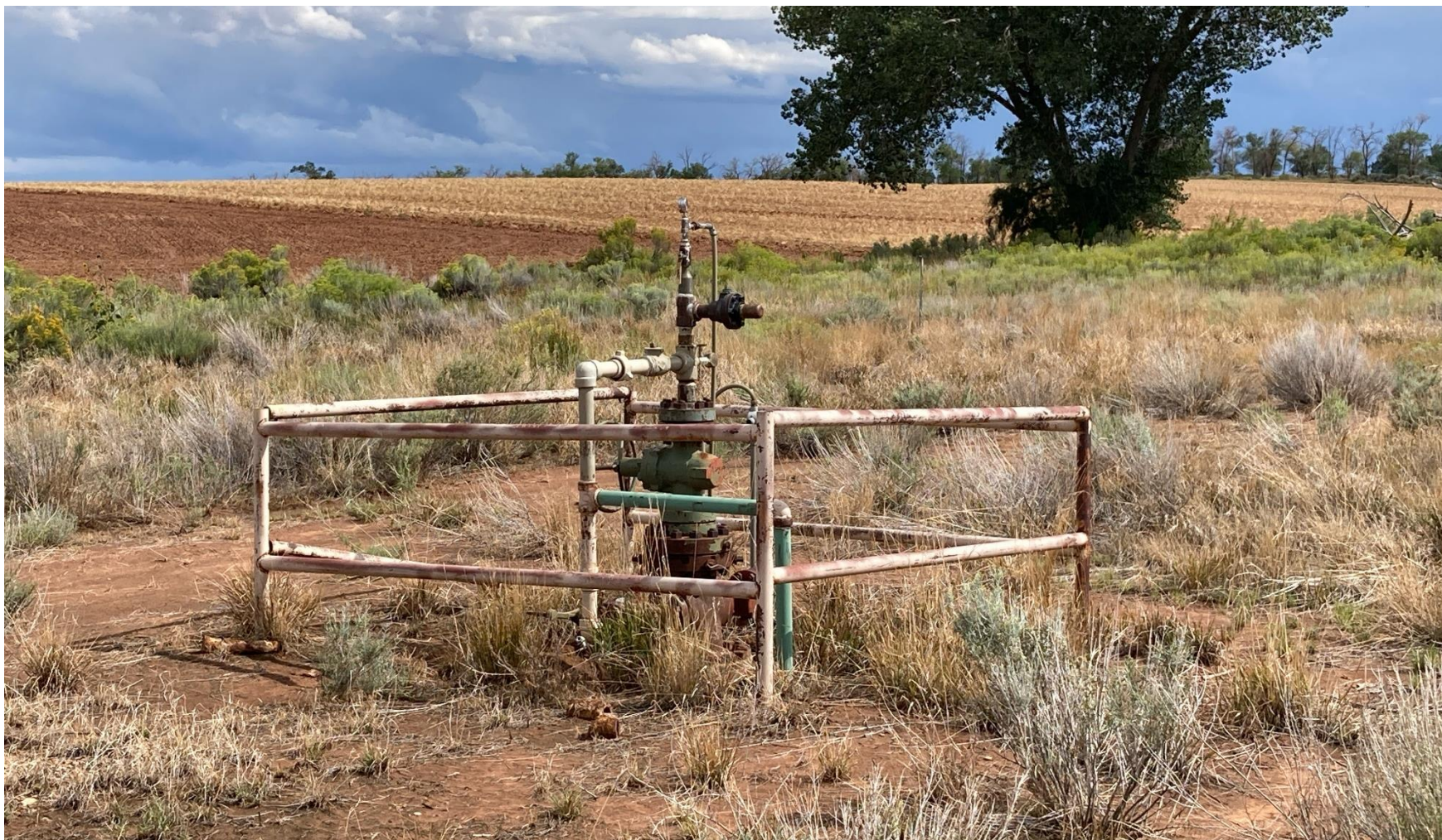
PHOTO 3: WELLHEAD AND EQUIPMENT/ WEEDS AROUND WELLHEAD NOT MAINTAINED. MAINTAIN WEEDS PER RULE 606.
