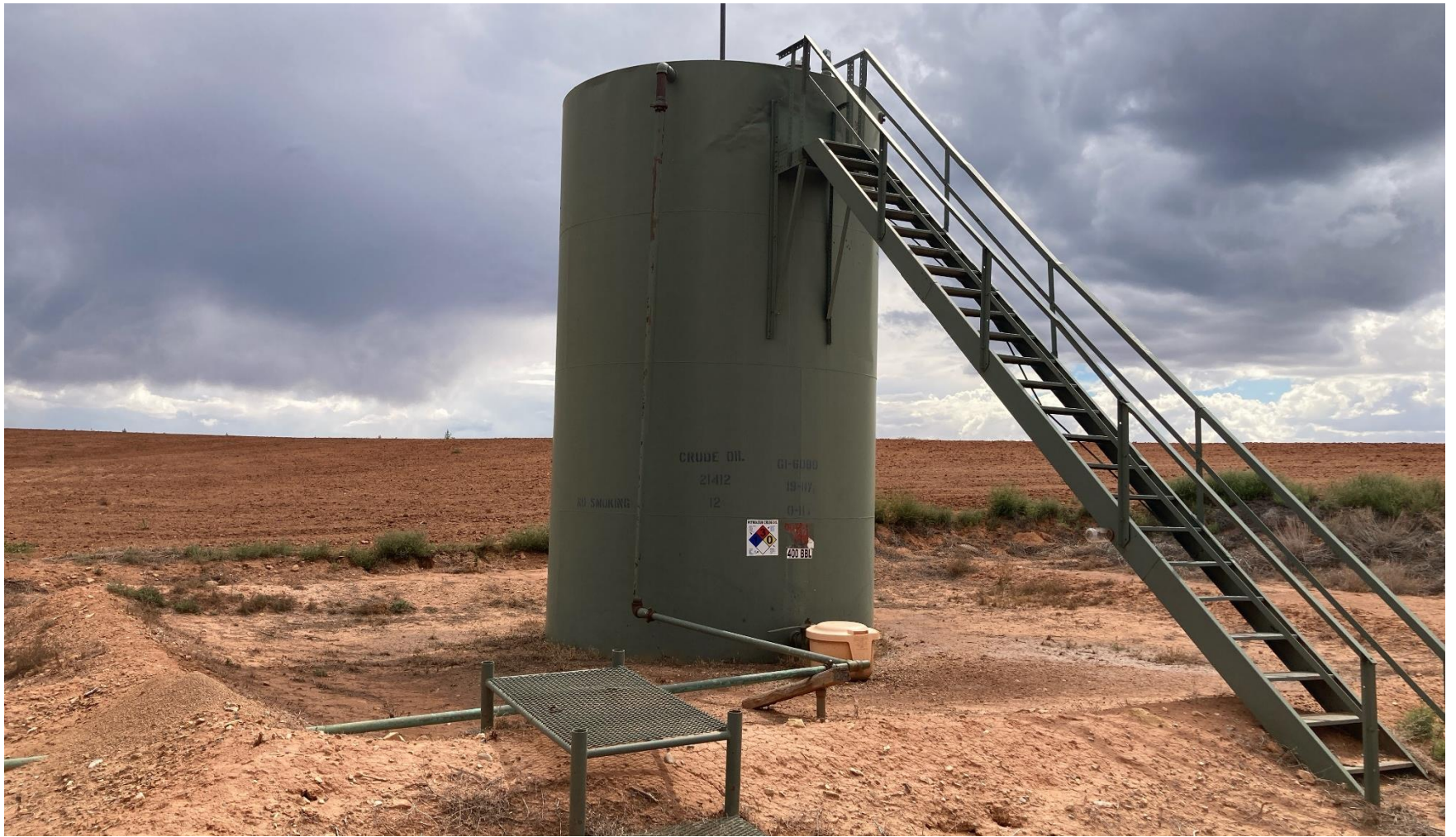
PHOTO 4: tank battery
