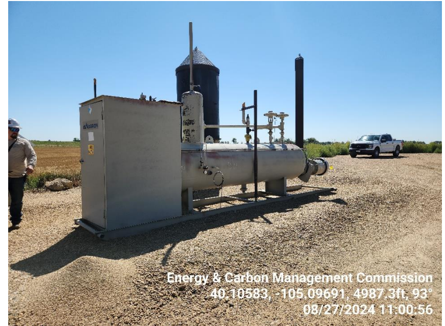
Photo 4 Horizontal Heated Separator
