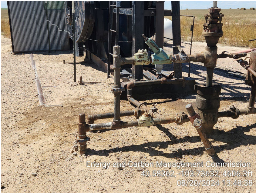
Photo 13 – Wellhead – Stained Soil
