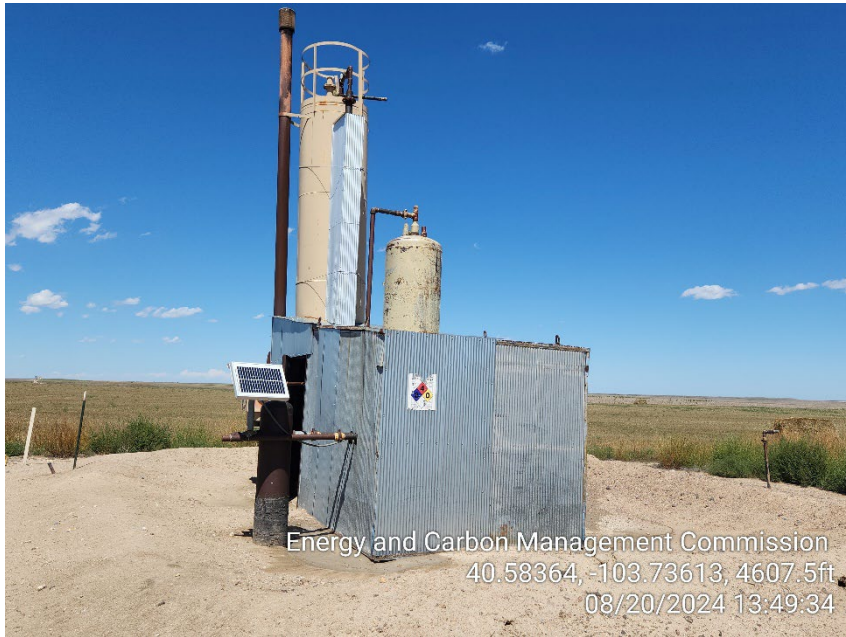
Photo 15 – Heater Treater
