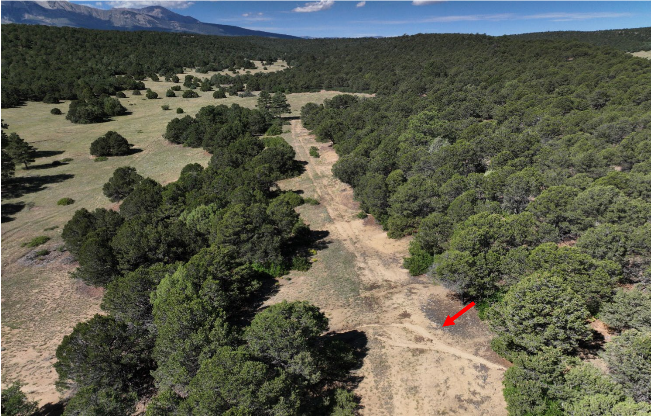
Photo 3. Drone aerial photo facing southwest along the access road. The area at the red arrow appears to have erosion issues.
