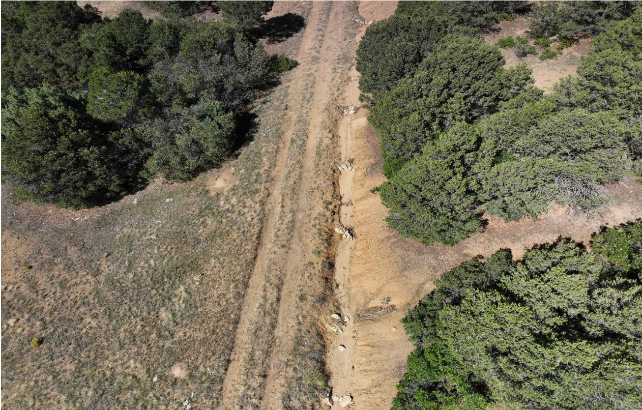
Photo 2. Drone aerial photo facing down toward the ditch along the access road. The check dams have fallen apart and the ditch is not stabilized.
