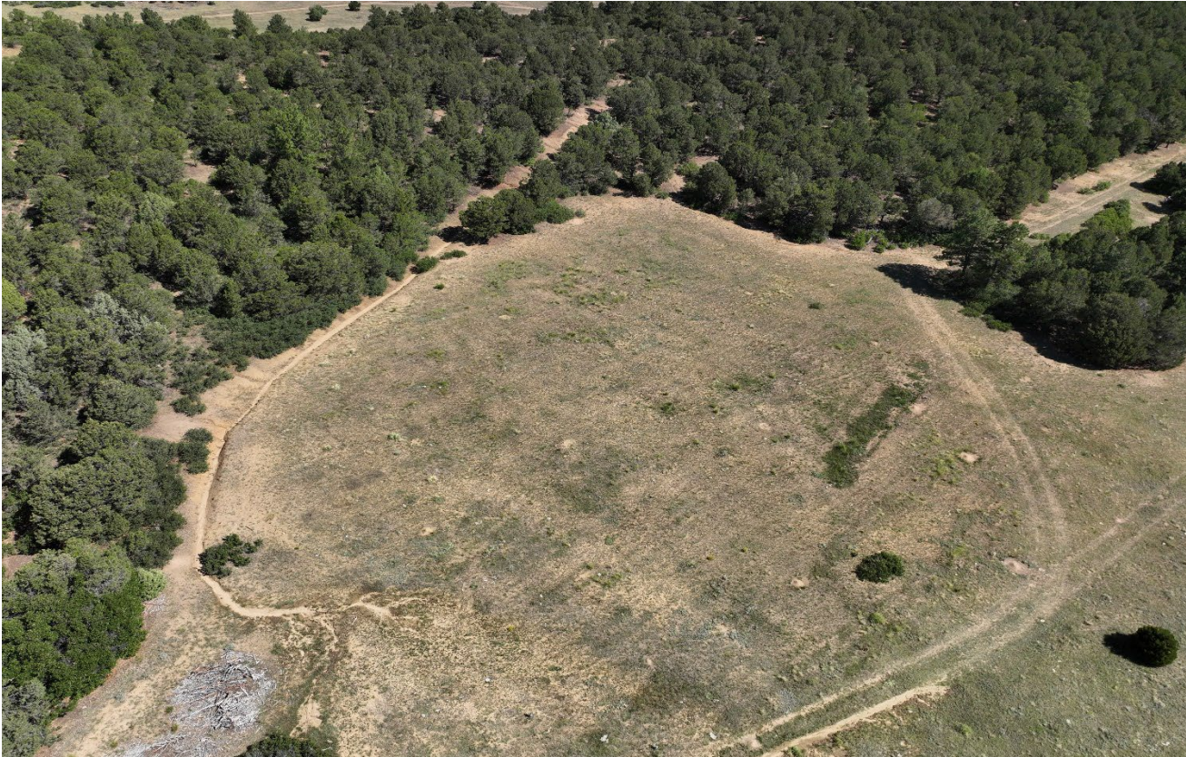
Photo 4. Drone aerial photo facing northeast toward the location. There is a perimeter run-on ditch along the northwest side of the pad that appears to be causing erosion.
